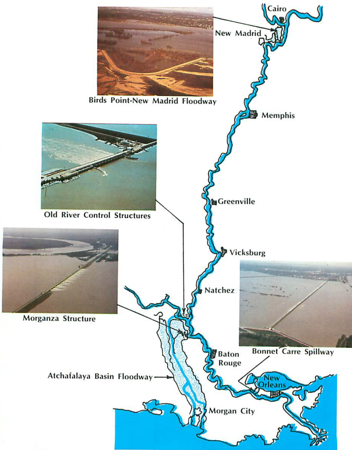
Figure 8. Control Structures and Floodways in Mississippi River and Tributaries Project
